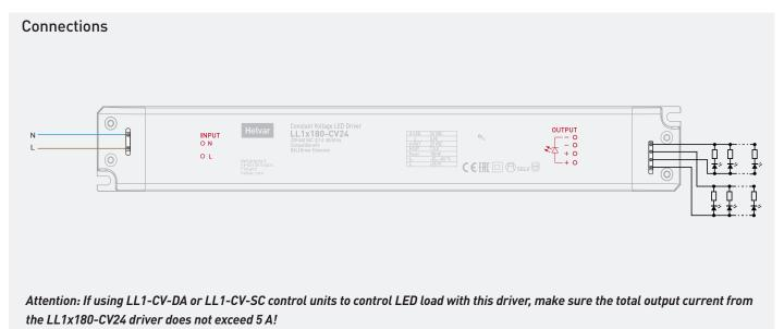
Note: Avoid using longer LED strips that 5 meters, the voltage losses grow substantial with long runs. In case of uneven brightness of LEDs in long strips, parallel connection of shorter strips is recommended.
